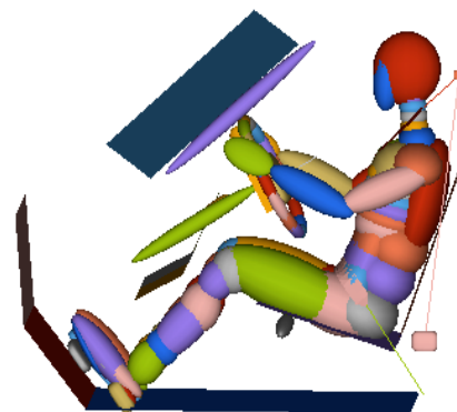
Figure 2: Simulation model for occupant restraint system
