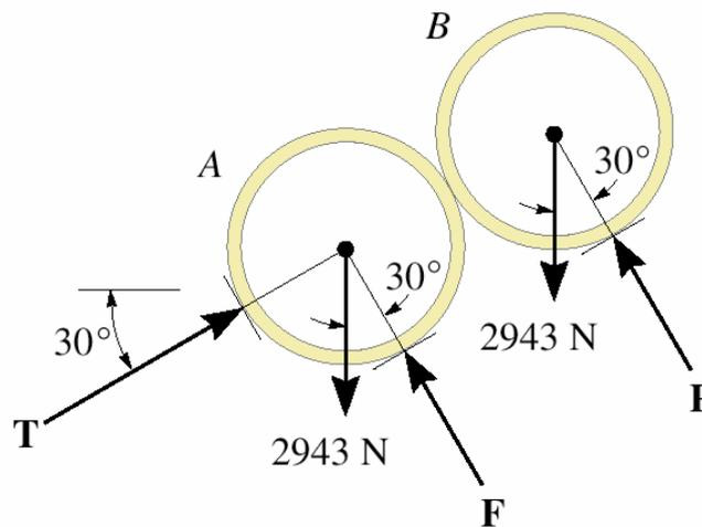
When pipes A and B are considered as one object, you neglect the reaction forces between them.
