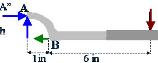
Effect of applied force acting on the spanner wrench
