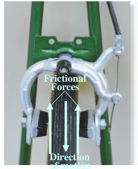
**Impending motion:** Impending motion refers to the state just before surfaces start to slip. In this case the static frictional force has reached its upper limit and is given by the equation:
