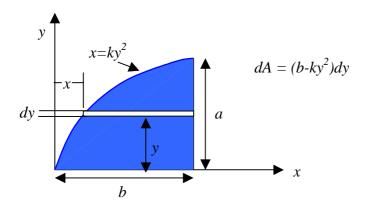
All parts of the differentia area element are the same distance from the x-axis
