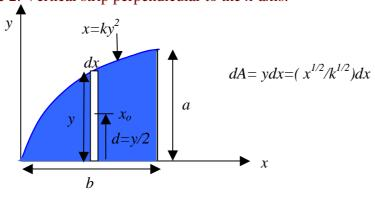
Since all parts of the element area are not at the same distance from the x-axis, we find the moment of inertia by considering the <u>differential area</u> about the x-axis:
