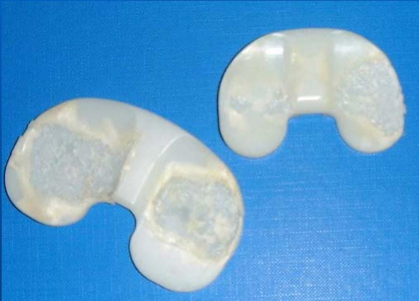
Most common failure in a TKR is due to the deterioration of the UHMWPE meniscal insert. This is due to geometric deformation, adhesive wear, surface pitting, 3 body abrasive wear, and most destructive - **DELAMINATION**
