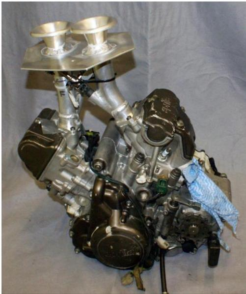
The engine in adjacent figure (figure 5), is one of the more demanding but interesting parts of the car. We have replaced 600 cc four cylinder engines for 550 cc two cylinder Aprilie. These engines are half the weight, more compact and have high torque from idle. Daniel Bartos and others have applied industrial software to try to develop an intake that feed both cylinders equally.
