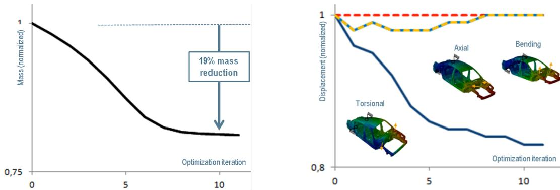
Figure 10 – Mass and stiffness constraints optimization iteration history for the free sizing optimization process
