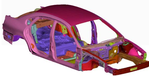
Figure 8 – Automotive finite element model considered for sizing optimization
