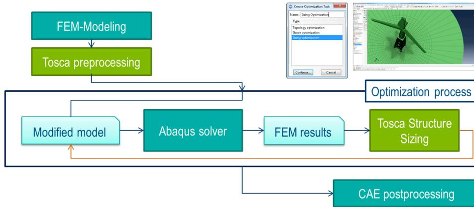
Figure 1 – Tosca Sizing process workflow
