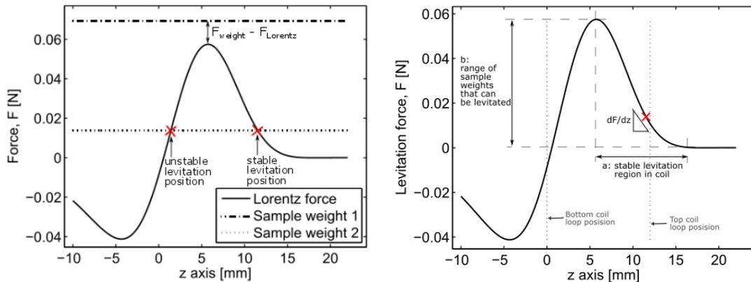
(a) Possibilities of stable, unstable and no levitation. (b) Effect of  $dF/dz$  on stability and the range of sample weights that can be levitated.
