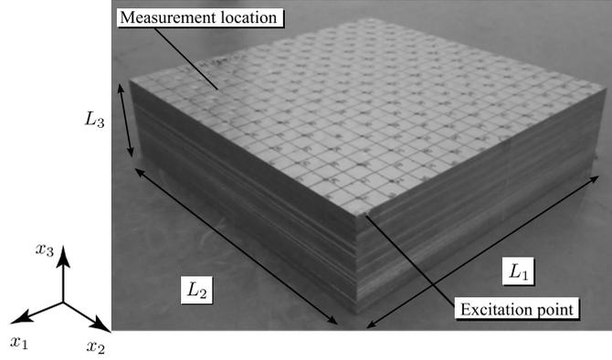
Figure 4: Photograph of the test specimen: laminated electrical steel sheets
