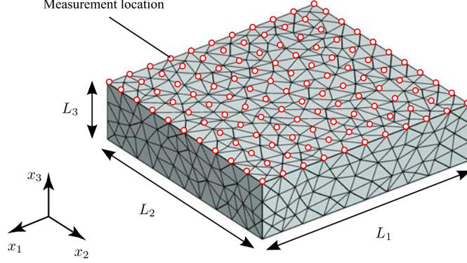
Figure 1: Numerical model with orthotropic material model
