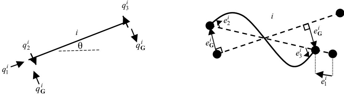
Figure 1: Generic 2D frame element  $i$  with second-order geometric nonlinearity (a) generalized stresses, (b) generalized strains
