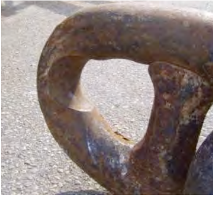
Figure 8: Adhesive (sliding) wear in the interlink zone.
