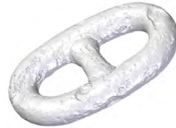
Figure 6: Computer model of chain link constructed from photogrammetric data [7].
