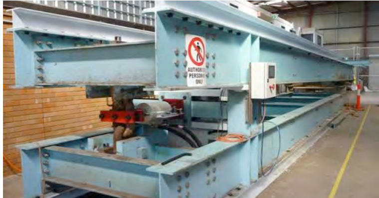
Figure 9: Wear rig at The University of Newcastle, Australia, showing 5-link chain set under cantilever-applied static axial load and hydraulic oscillatory lateral loading system.
