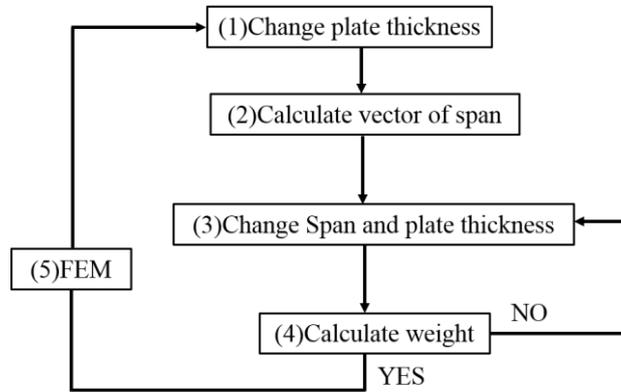
Figure 4: flow of optimization method
