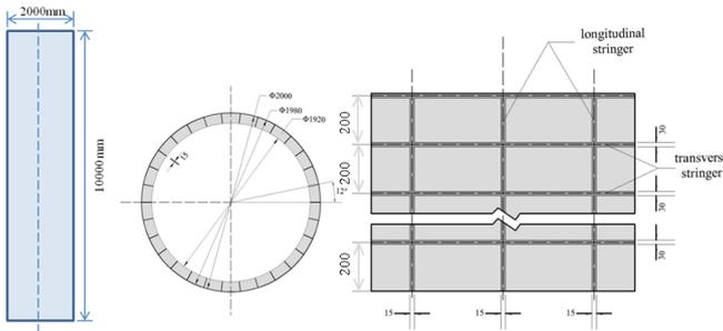
Figure 2: Typical stiffened cylindrical shell structure
