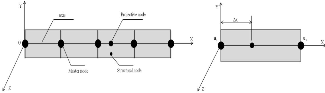
Figure 1: Principle of the model reduction method
