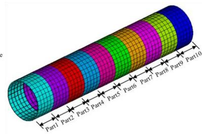
Figure 3: FEM model of the cylinder structure
