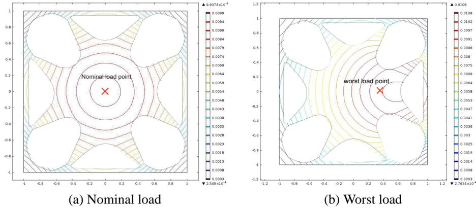
Figure 9: Out-of-plane deformation distribution for deterministic optimum configuration
