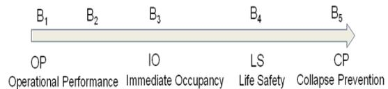
Fig.2 Damage levels and performance levels
