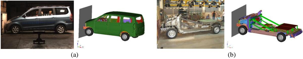
Figure 2: Physical model and FE model under 100% frontal impact: (a) full-scale vehicle; (b) simplified frontal impact model
