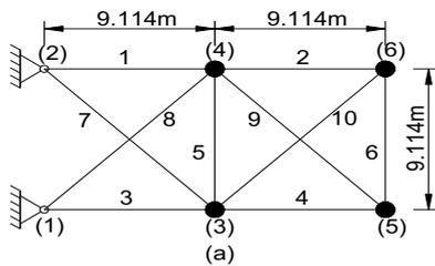
Figure 1: (a) Model of 10-bar truss
