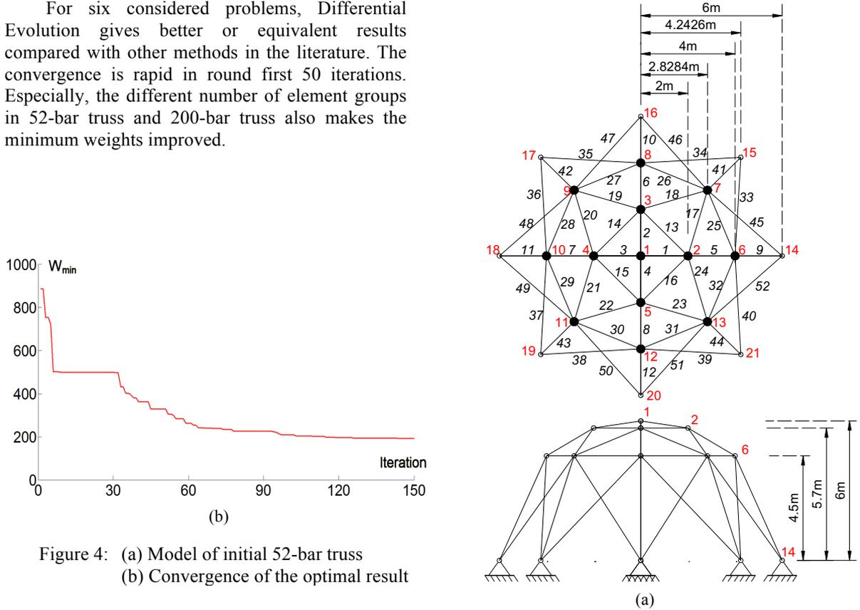
Figure 4: (a) Model of initial 52-bar truss
