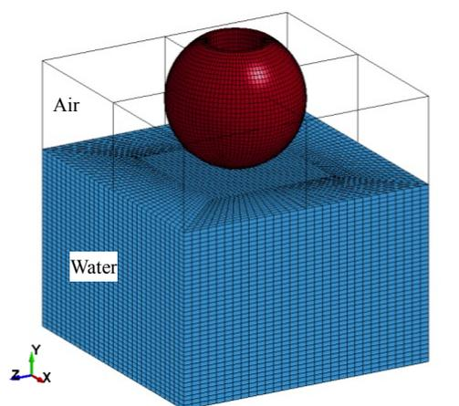
Figure 3 Three view of water impact model including air and water domain
