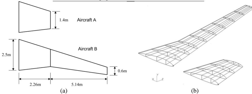
Figure 2: Planform and finite element models of the two aircraft wings
