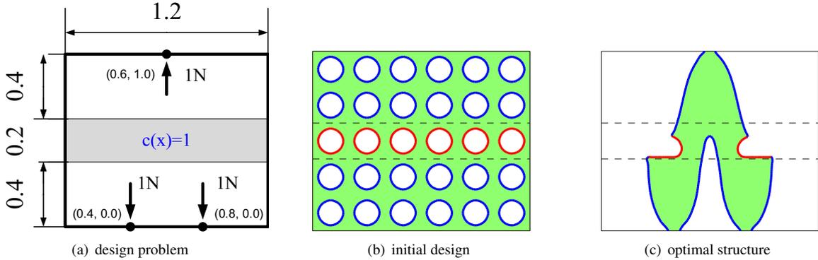
Figure 2: Design problem, initial design, and optimal structure.
