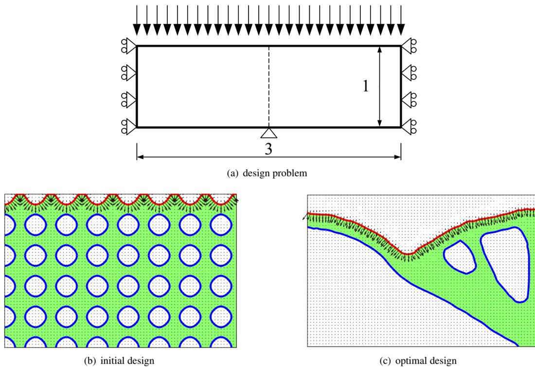
Figure 3: Design problem, initial design, and optimal design.
