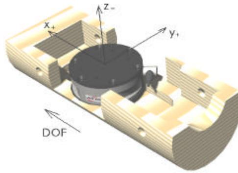
**Figure 2** The 9105-ISA-Delta 6-component load cell, fitted onto the fuselage insert
