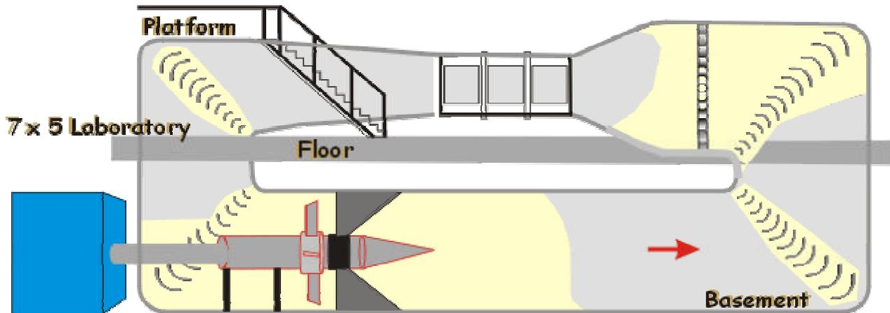
Figure 1 The 7x5 Low Speed Wing Tunnel
