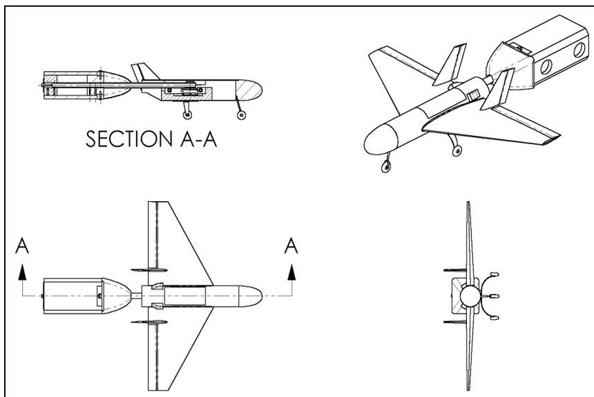
**Figure 4** Model of *Brumby* Mk II as fitted onto the pitch-yaw mechanism
