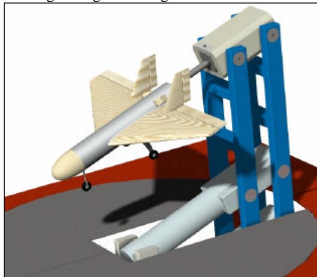
**Figure 3** CAD picture showing the *Brumby* model in the Wind Tunnel
