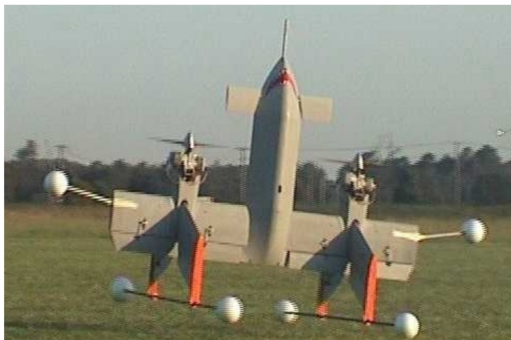
Figure 4 T-Wing Technology Demonstrator Vehicle undergoing preliminary hover flight tests
