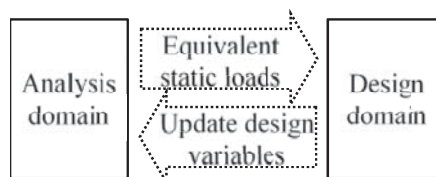
Figure 2: Schematic view of the equivalent static loads method
