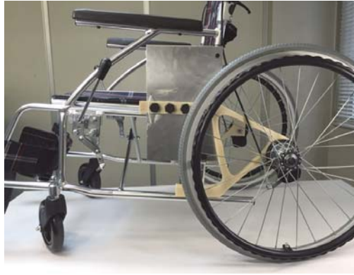
Figure 8: Wheelchair in which a suspension is installed
