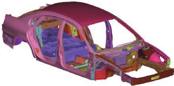
Figure 8 – Automotive finite element model considered for sizing optimization
