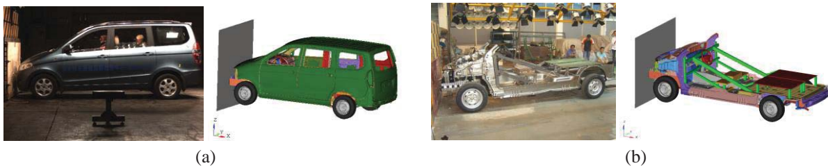
Figure 2: Physical model and FE model under 100% frontal impact: (a) full-scale vehicle; (b) simplified frontal impact model
