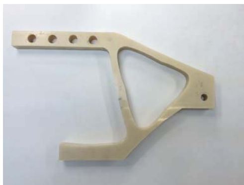
Figure 7: Suspension manufactured by a milling machine
