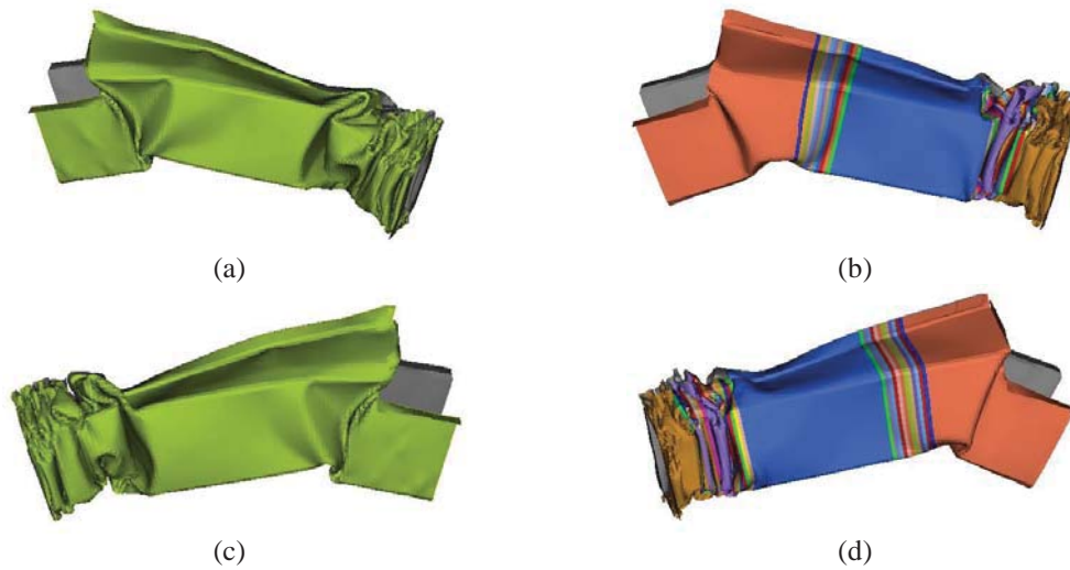
Figure 15 Comparison of the numerical result before and after optimization: (a) Left FLB of baseline design; (b) Left FLB of optimal design; (c) Right FLB of baseline design; and (d) Right FLB of optimal design
