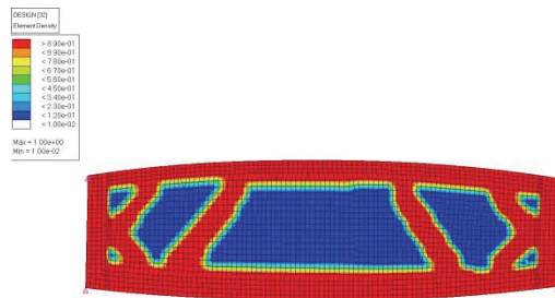
Figure 14 : Topology optimization plot for Rib 10
