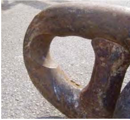
Figure 8: Adhesive (sliding) wear in the interlink zone.
