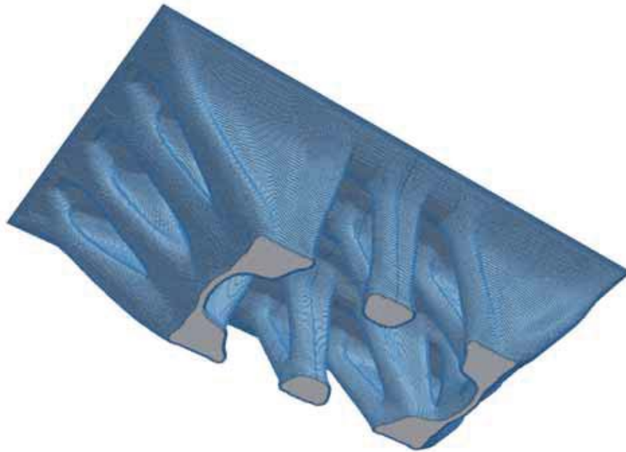
Figure 4: Full 3D structure optimized using the coating approach. The coating material is rendered at 35% transparency to visualize the internal base structure.
