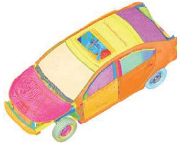
Figure 3: Full-size finite element model of frontal impact simulation
