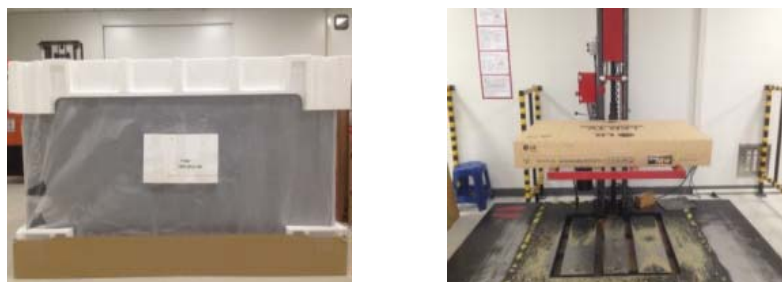
Figure 6: Verification test of the results : a) Pilot package, b) Drop test
