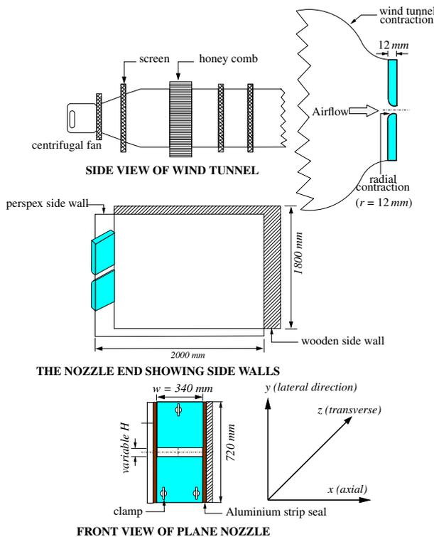
Figure 1: Schematic of the plane jet facility.
